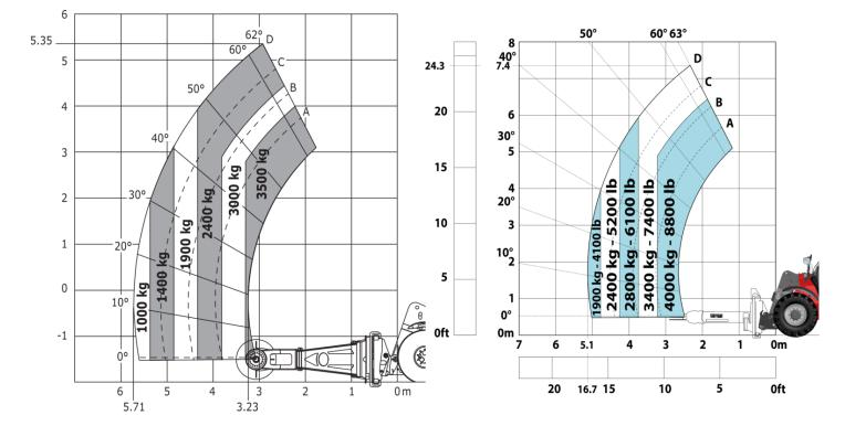
Machine on tyres with tyre handler TH 49 (Metric)
