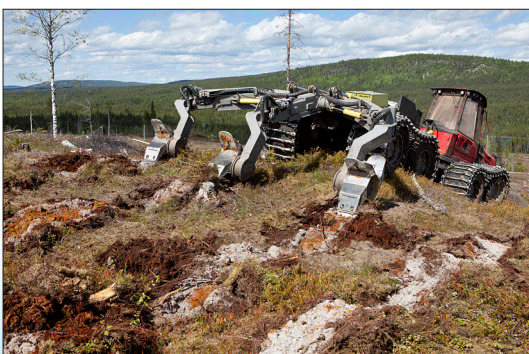
Scarification with the M36.b gives plants and seeds the best possible start for growth and survival whatever the terrain.
