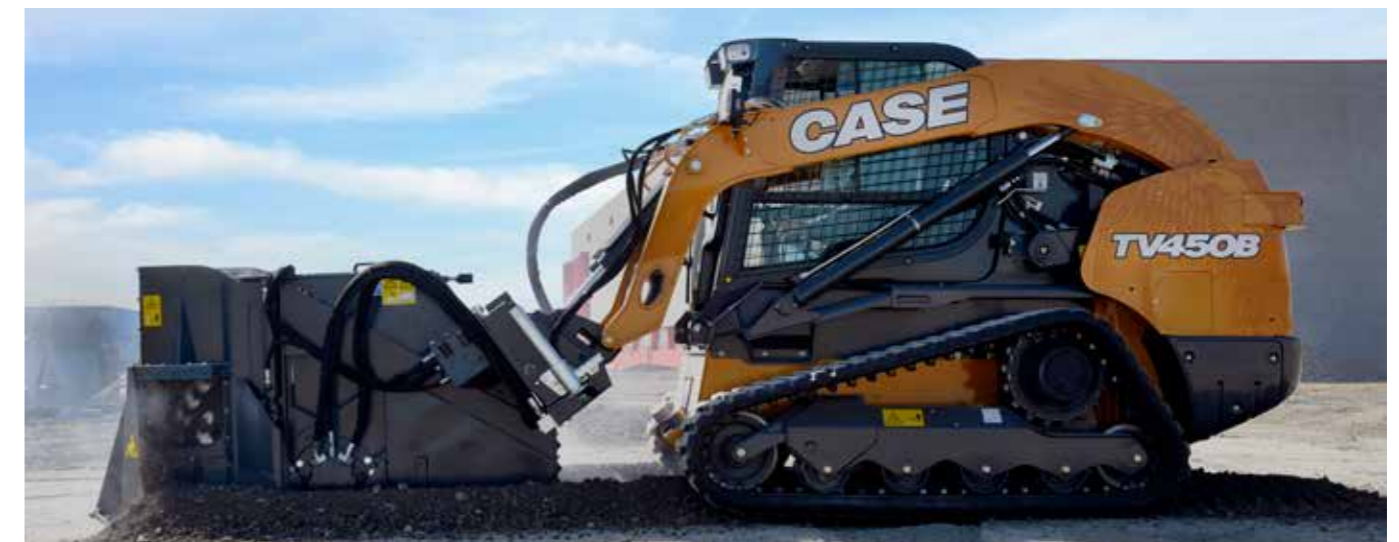
Additional Counterweight to increase ROC
