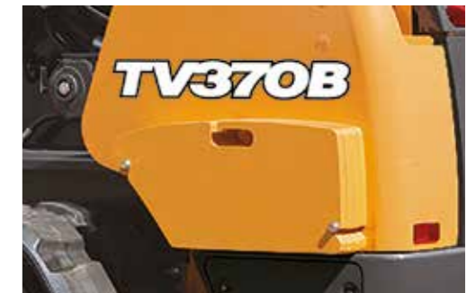
Additional Counterweight to increase ROC
