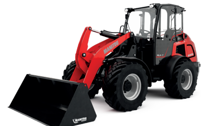
MLA Articulated Loader with z-bar linkage* 2
